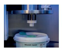
The automatic filling system is lowered and the dispensing nozzle penetrates the seal valve
