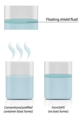
This floating shield fluid is immiscible with formalin, having a lower specific gravity, and covers the top surface to form a protective film. This proprietary fluid is nontoxic and inert to biospecimens: if the container is agitated, the floating layer quickly reforms.
