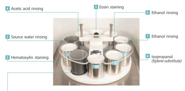
Preheated (37°C) FineFix solution for the simultaneous specimen fixation, dehydration and clearing. FineFix is a formalin-free, ethanol-based (70%) solution, ideal for histological applications and molecular studies.
