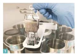
Position the slide rack over the FineFIX processing vessel.
