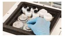
5 Place the chuck into the mold.
