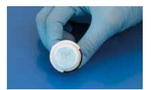
4 After 60 seconds, the specimen is ready for section cutting.
