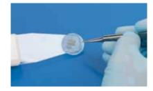
Position the specimen on the lens paper. Check its orientation.
