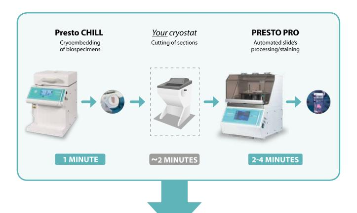
From fresh biospecimens to six stained frozen sections of permanent-like quality in less than **10 minutes**.
