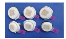
Each mold can be separately timed through the built-in control panel. Up to **6 samples** can be frozen in parallel or in sequential order in less than **4 minutes**.
