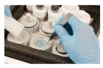
3 Gently slide the specimen, paper side down, into the mold. Add the cryoembedding compound, the chuck and the heat extractor.
