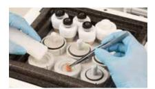
3 Transfer the specimen to the bottom of the mold.
