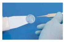
1 Wet both sides of a small section of lens paper with the cryo-embedding compound.
