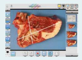
MacroPATH macro digital imaging system for automatic, rapid documentation of all the grossing steps of surgical pathology specimens. State-of-the-art digital camera: - Resolution: 20.1 Mpx (image size: 5184×3888 px) - Magnification: 30x optical - Automation: autofocus, auto-light adjusting, auto WB. - Supplemental lighting: built-in LED
